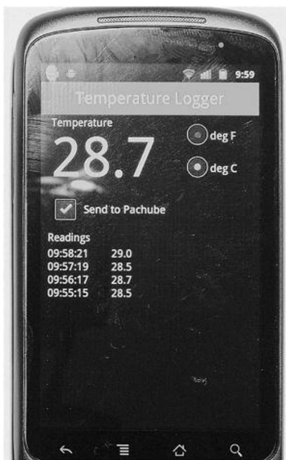
**Figure 5-2** The Android Temperature Logger app
