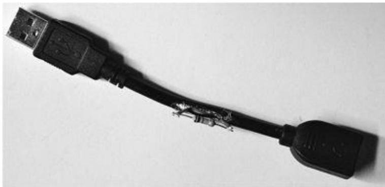
**Figure 2-19** Fixing the resistor in place
