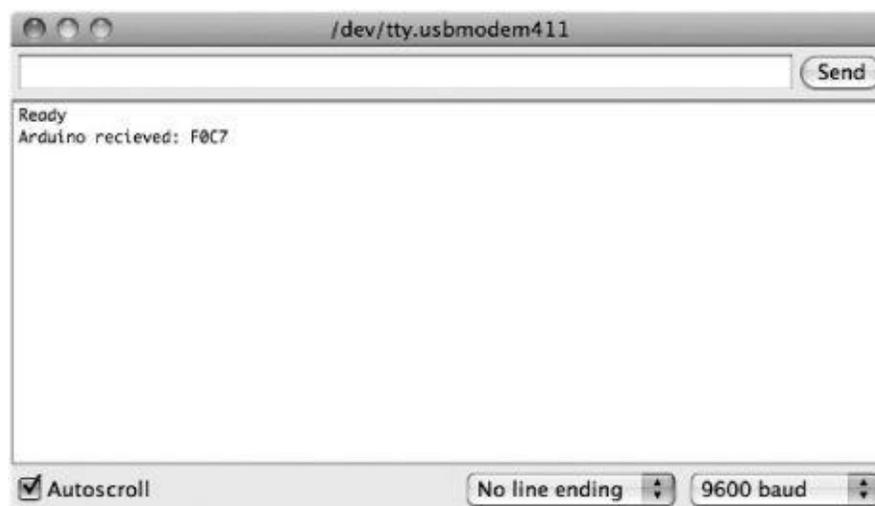
**Figure 7-17** The Serial Monitor
