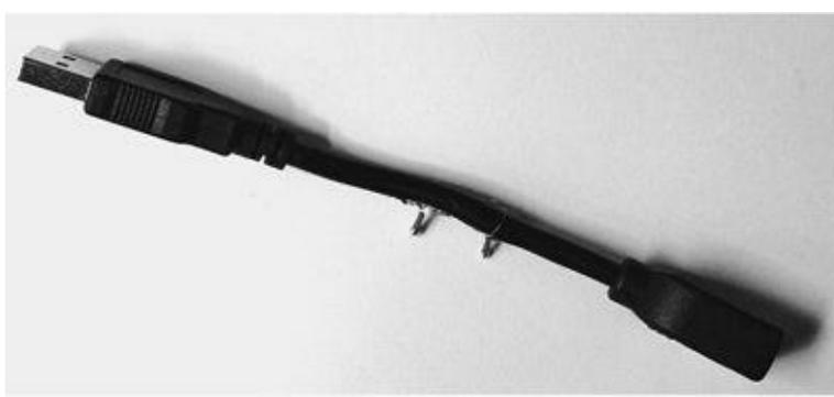
**Figure 2-18** Making a USB nonpowered lead
